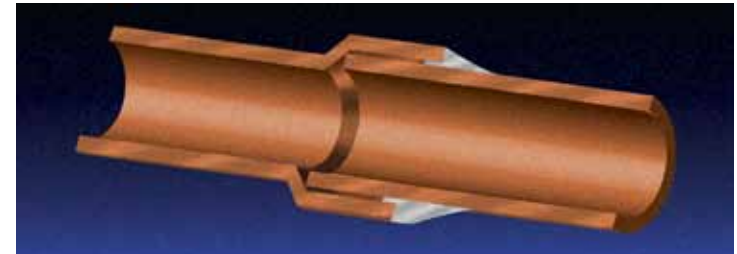
Improper alloy flow does not penetrate into the joint and produces a weak bond.
