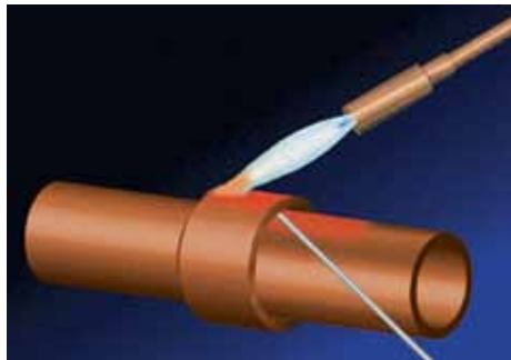
Once the assembly has reached brazing temperature the filler metal is applied.
